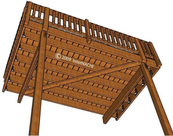
Underside Diagonal Bracing
